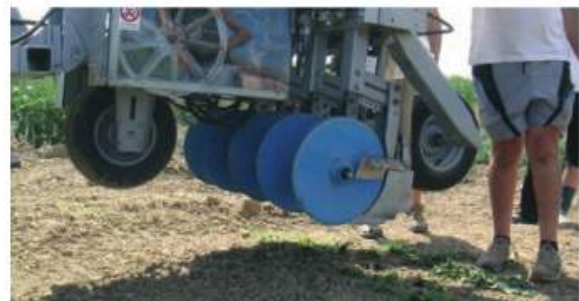
Photo 1 Fully automated transplanting machine: details of the double disk coulters used for transplanting single plants into an existing turf.
