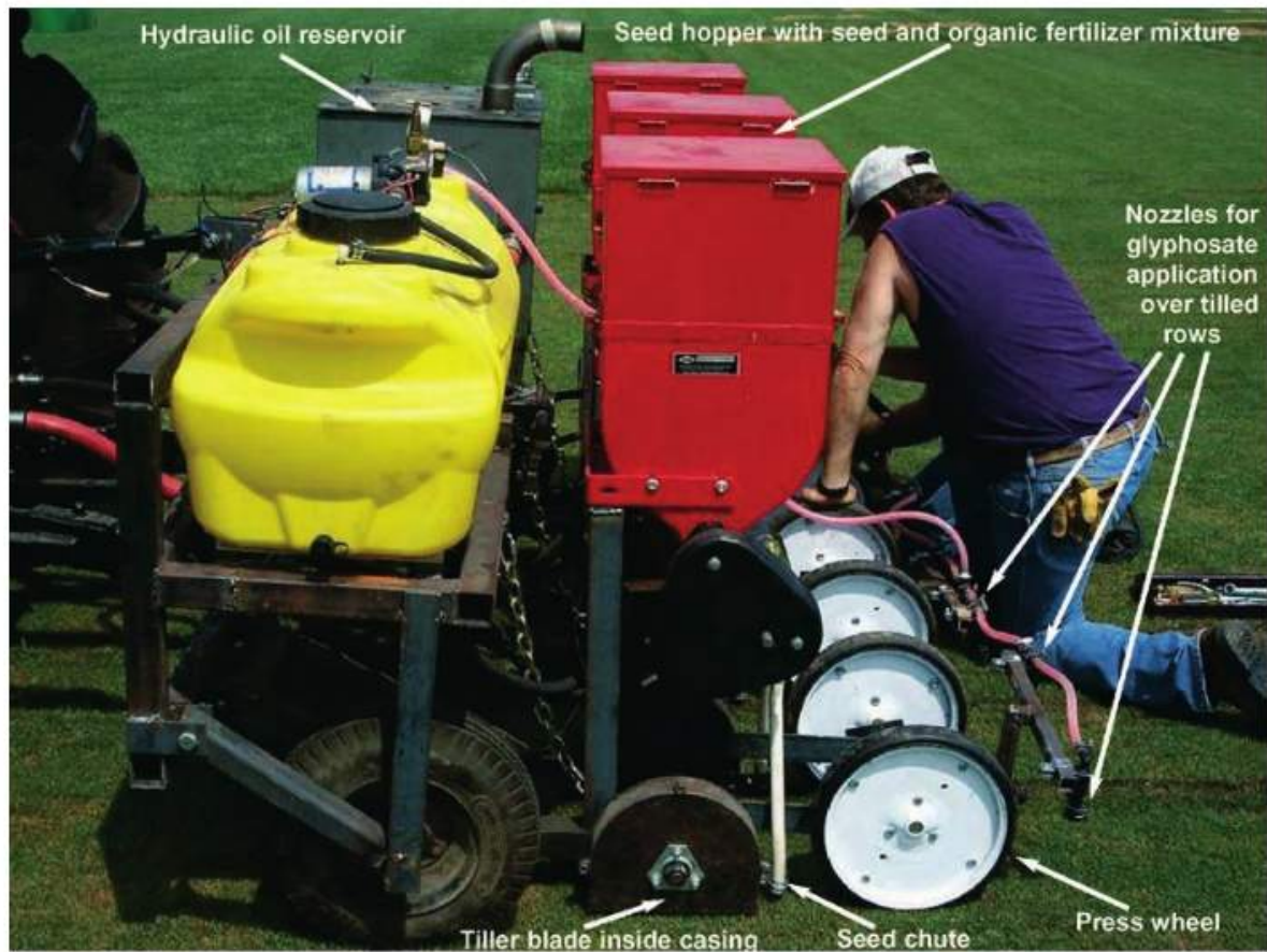
Figure 1 The strip seeder and its components that were used to convert a perennial ryegrass turf to seeded 'Riviera' bermudagrass (Fry et al., 2007. Strip seeding: A new approach for converting cool-season turf to warm-season grasses. USGA Turfgrass and Environmental Research Online 6(4):1-6).
